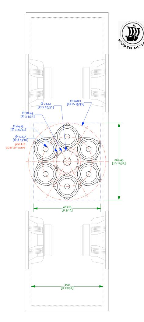
Hexagonal CHN-40 Array 0V7 4 x Mark Audio CHN-40 + Tweeter 19-december-2022 | Sheet 0 – 18mm plan designed by Scott Lindgren | drawn by dld © 2022 Woden Design | licenced use only
